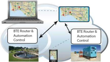
The BTE Router is an intelligent device capable of managing its own day-to-day operations and raise flags when exceptions occur. BTE's CloudTrak monitors the summary status of all network elements and provides the navigation to assist operations personnel in quickly identifying and correcting the endpoints in fault.
